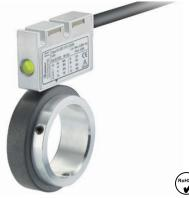
Thanks to its installation depth of only 16 mm, the bearingless magnetic rotary encoder RLI20, comprising a magnetic ring and sensor head, is ideally suited for plants and machinery where space is very tight. The non-contact measuring principle allows for error-free use even under harsh environmental conditions, as well as ensuring a long service life.
